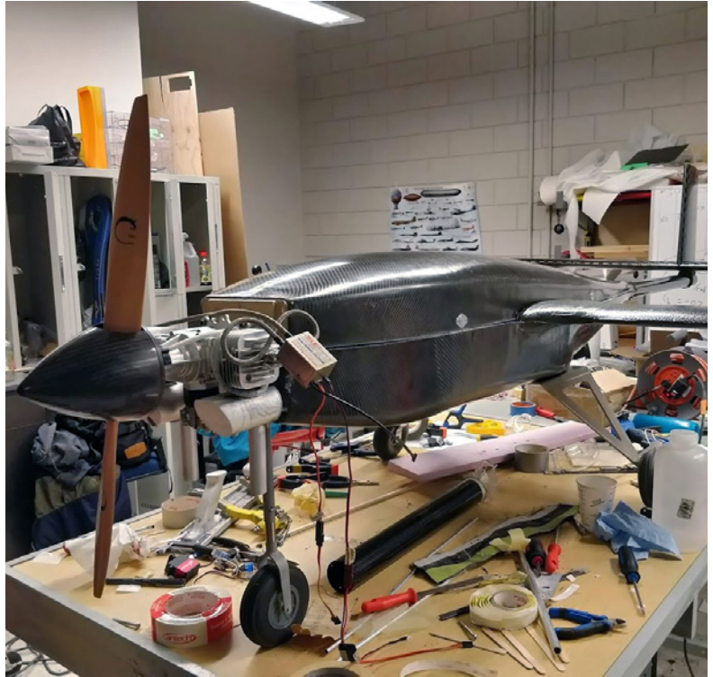
Landing gear and propulsion assemblies mounted to the fuselage during manufacturing. Materials were provided by ICARUS Aerospace.
